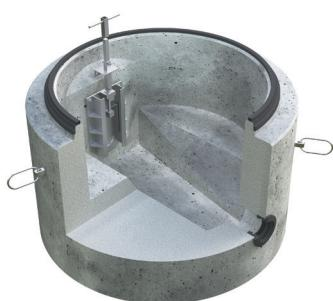
The discharged quantities from the ACO Stormbrixx block storage are adjusted and controlled via the ACO flow restriction manhole, a manhole structure made of reinforced concrete with integrated flow restriction valve for individual reduction of the discharge pipe crosssection. In this way, collected surface water is discharged into the sewer in a controlled way, without overloading it.
