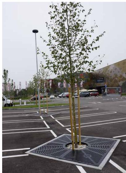
**Massive cast iron tree grates** provide normal living conditions for trees – even in a completely urban environment – because despite waterproof ground they enable air and water supply for the root system and prevent damage due to parked vehicles.
